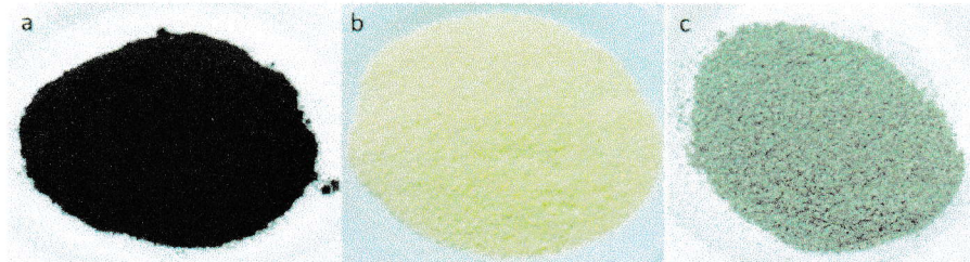
Figure 1. a) Rubber particle (GTR), b) HDPE after grinding, c) HDPE and GTR particle after mixing.
